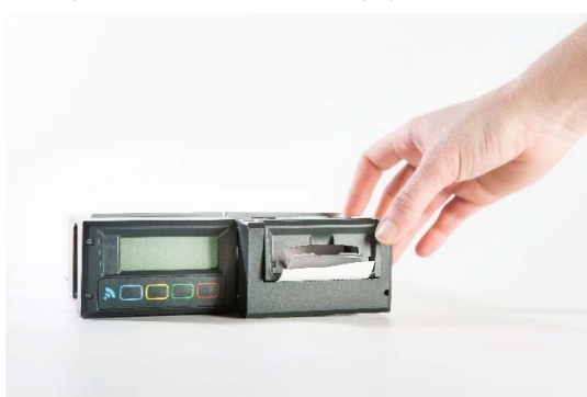
4.) After changing the paper please install the printer with the flap open.
