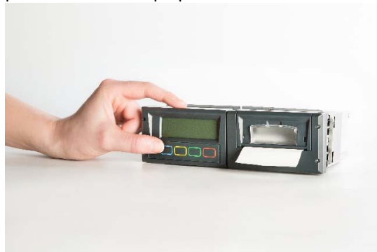
6.) Test if the paper roll is properly replaced by printing any ticket.
