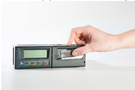
5.) Close the flap only after the printer is fully inserted.
