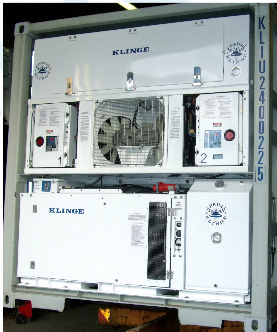
NMR-262—Nose-Mount Dual Redundant Container System: Two Full-Capacity Refrigeration Integral Genset for back-up power supply
