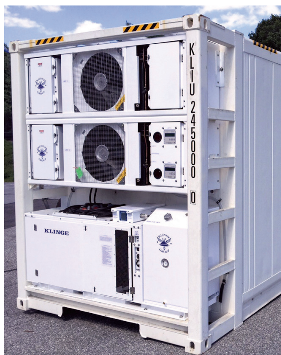
NMF-372—Deep Freezer Dual Redundant Container System: Two Full-Capacity -65°C Freezer Units, Integral Genset for back-up power supply
