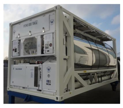
The TCR-262 is based on the same platform as its popular air-cooled Dual Refrigeration System NMR-262 Unit used for transport of such items as organic peroxides and self-reactive substances. The TCR-262 utilizes a heat transfer fluid to cool liquid cargo in tank container features two refrigeration with systems two independent microprocessor thermostats controllers that communicate with each other to provide 100%
