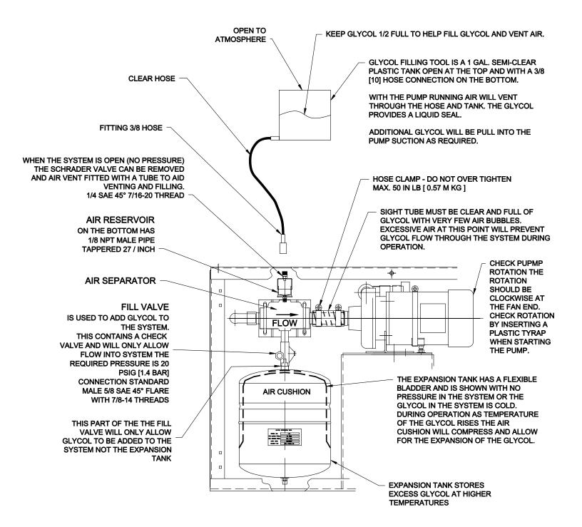
ADDING GLYCOL SYSTEM AND VENTING AIR WITH NO PRESSURE IN THE SYSTEM MODEL TCR-104-04 THRU 09
